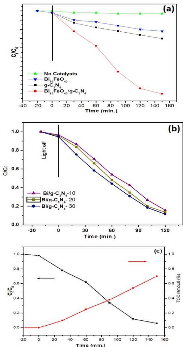
Fig. 3. (a) The 2-CP photo-degradation with different photocatalysts under visible light; (b) The 2-CP photo-degradation with Bi/gC<sub>3</sub>N<sub>4</sub> composites of 10,20,30 wt%. (c) The mineralization of 2-CP using Bi<sub>25</sub>FeO<sub>40</sub>/g-C<sub>3</sub>N<sub>4</sub> composite under visible light.
