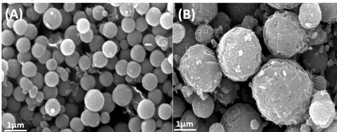
Fig. 2. SEM image of the as-prepared  $\text{Bi}_{25}\text{FeO}_{40}$  microspheres and  $\text{Bi}_{25}\text{FeO}_{40}/\text{g-C}_3\text{N}_4$  microspheres
