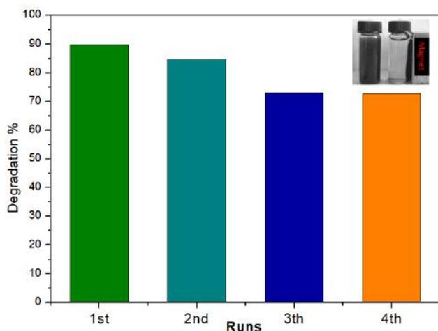
Fig. 5. The stability of the Bi/g-C<sub>3</sub>N<sub>4</sub> composites after 4 recycles
